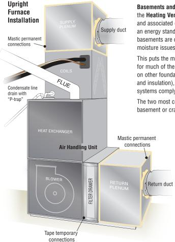
Basements and crawlspaces are often used as a location for the Heating Ventilation and Air Conditioning (HVAC) system and associated ductwork, although not always ideal from an energy standpoint. Vented crawlspaces or unconditioned basements are cold in the winter and often experience moisture issues in the summer.
