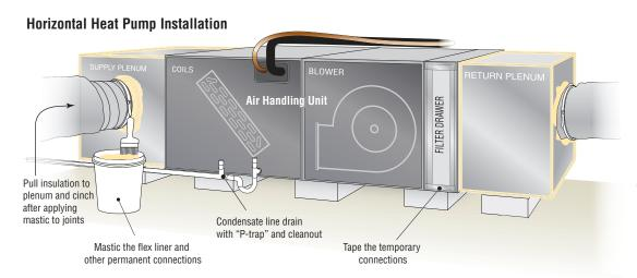
Whether a heat pump or a fuel-fired furnace, foundation-located HVAC systems need proper attention to details such as: adequate drainage for water condensation from the evaporator coils, mastic sealant on permanent joints of the air handler unit and ductwork, taped seams of temporary enclosures such as the filter drawer and attention to regular maintenance needs.
