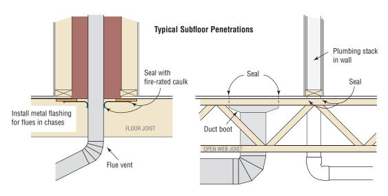
Different floor assemblies may provide unique challenges but the end result is the same - seal all cracks and penetrations
