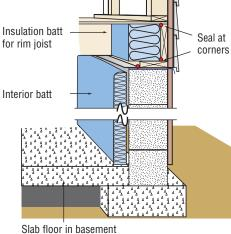
6 mil polyethylene and laps up foundation wall 6 inches
